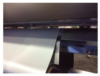
tendency may be to increase the heat setting to dry the ink. This may cause the magnetic base to soften, and the heavy weight of the stock may cause it to stretch. It is best just to use lower heat and allow the ink more time to air dry.
