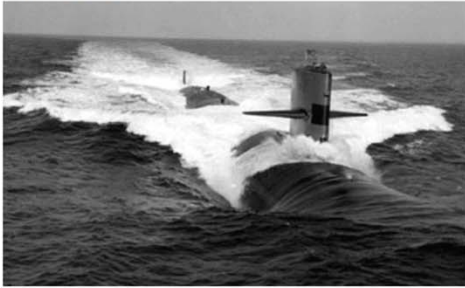
Two early nuclear-powered electric drive submarines: USS Tullibee (SSN-597, top), and USS Glenard P Lipscomb (SSN-685, bottom). Immature electric-drive technology in the 1960s and 1970s limited the performance of these boats in comparison to their mechanical-drive counterparts.
