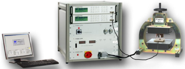
Figure 3. Typical hysteresigraph including a yoke structure, search coils for detecting the magnetic field, fluxmeters and power supply, computer control system and software.
