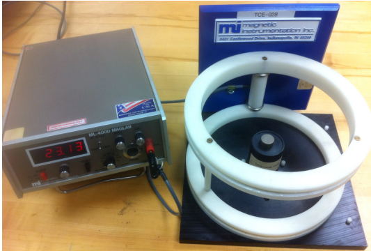
Figure 6. Arrangement of a Helmholtz coil set mounted horizontally and an integrating fluxmeter.
