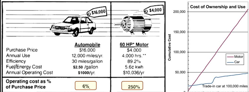
**Figure 1. First Cost is not the Last Cost**
