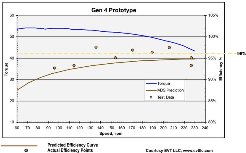
(Predicted Efficiency curve as illustrated by Motor Development Software, University of Glasgow)
